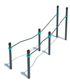
The complex consists of six vertical columns of different height, multi-width parallel bars 1790 mm in length and inclined parallel bars 1790 mm in length. The distance between the multi-width parallel bars is 598 mm at the narrow end and 1198 mm at the wide end. Total width difference for the parallel bars is 600 mm. The difference between the lowest and highest point of the inclined parallel bars is 466.3 mm. The structure is secured together with siluminium clamps. Weight - 150.20 kg.
